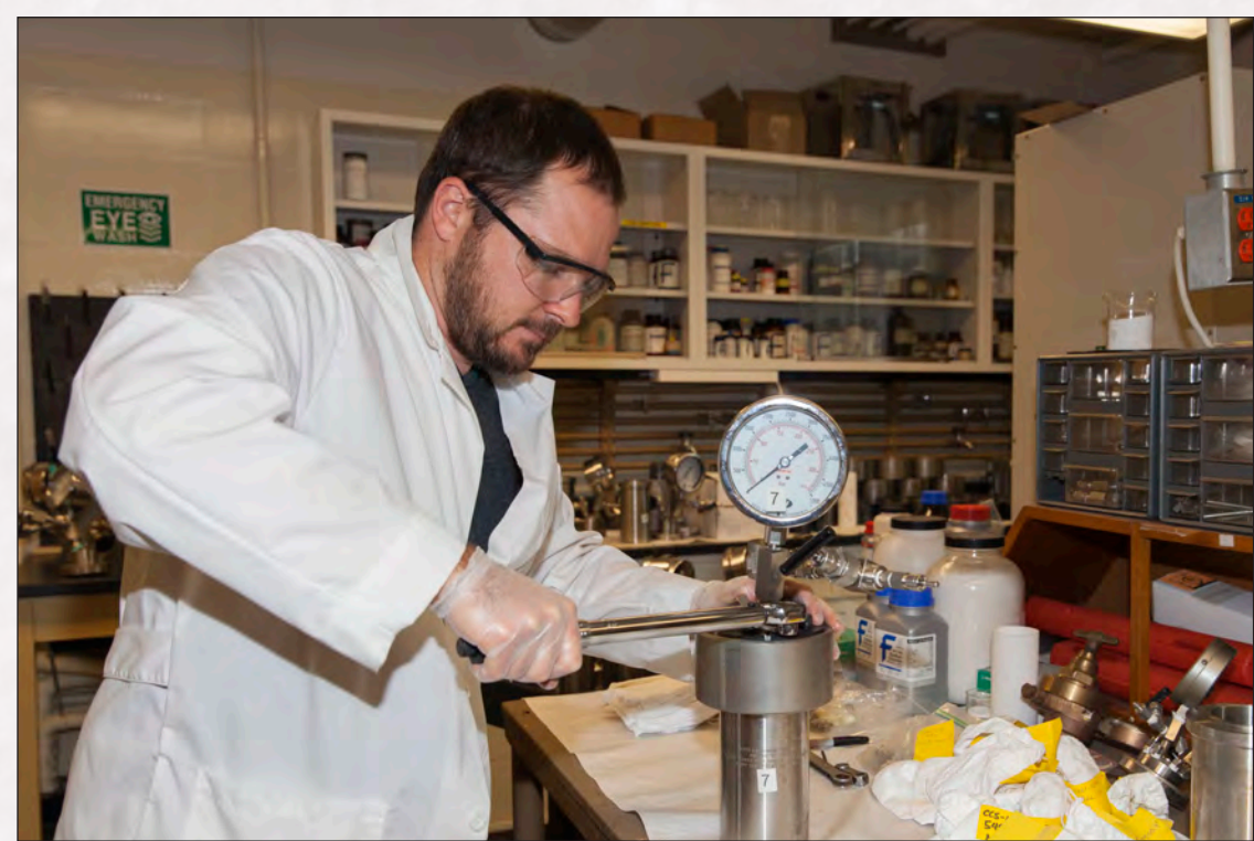
Figure 4. Preparing Parr pressure vessel for five month CO 2 -brine-rock reaction experiment.
